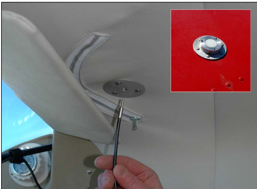
Figure 4. Uplinking Teflon port viewed from inside the cabin with the fiber optic tip ready for insertion. The tip fits into ball bearing detents for both up- and down-looking ports. The inset shows the port as it appears on the outside of the skin. This port measures about 4 cm across. The annular space of metal and raised design prevent the port from receiving reflected light.
