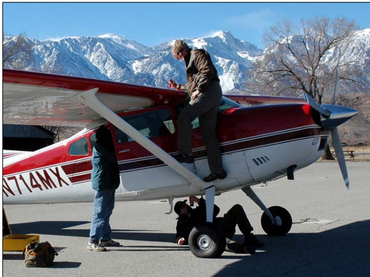
Figure 2. Cessna 185 equipped to fly non-imaging spectrometry. Activities include removing the cap from the uplooking Teflon-covered port (wing), mounting the downlooking foreoptic (belly), and securing the spectrometer in place (through door).
