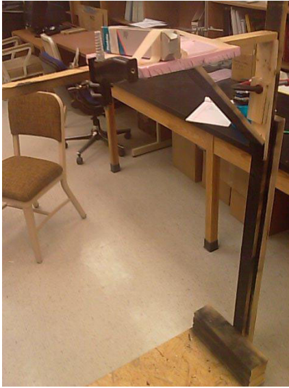
Figure 6. Shows the mounting stand with the pistol grip in which the fiber optic cable of the spectroradiometer is inserted. (Spectroradiometer is not shown)
