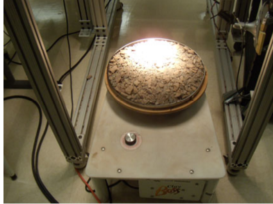
Figure 4b. Rotating pan of copper ore, particle size < 30 mm.
