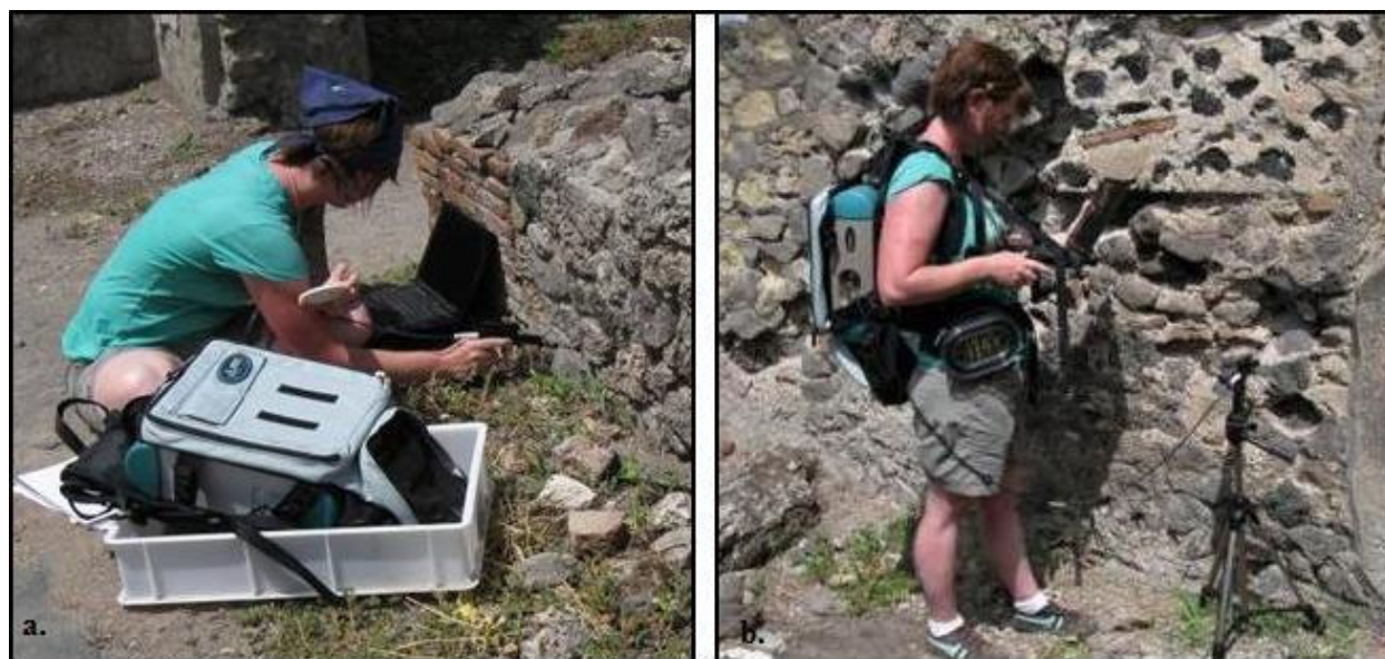
Figure 3: Data collection with the FieldSpec® 3. a. Hand-held configuration; b. Tripod mount configuration. Photos by Philip Murgatroyd
