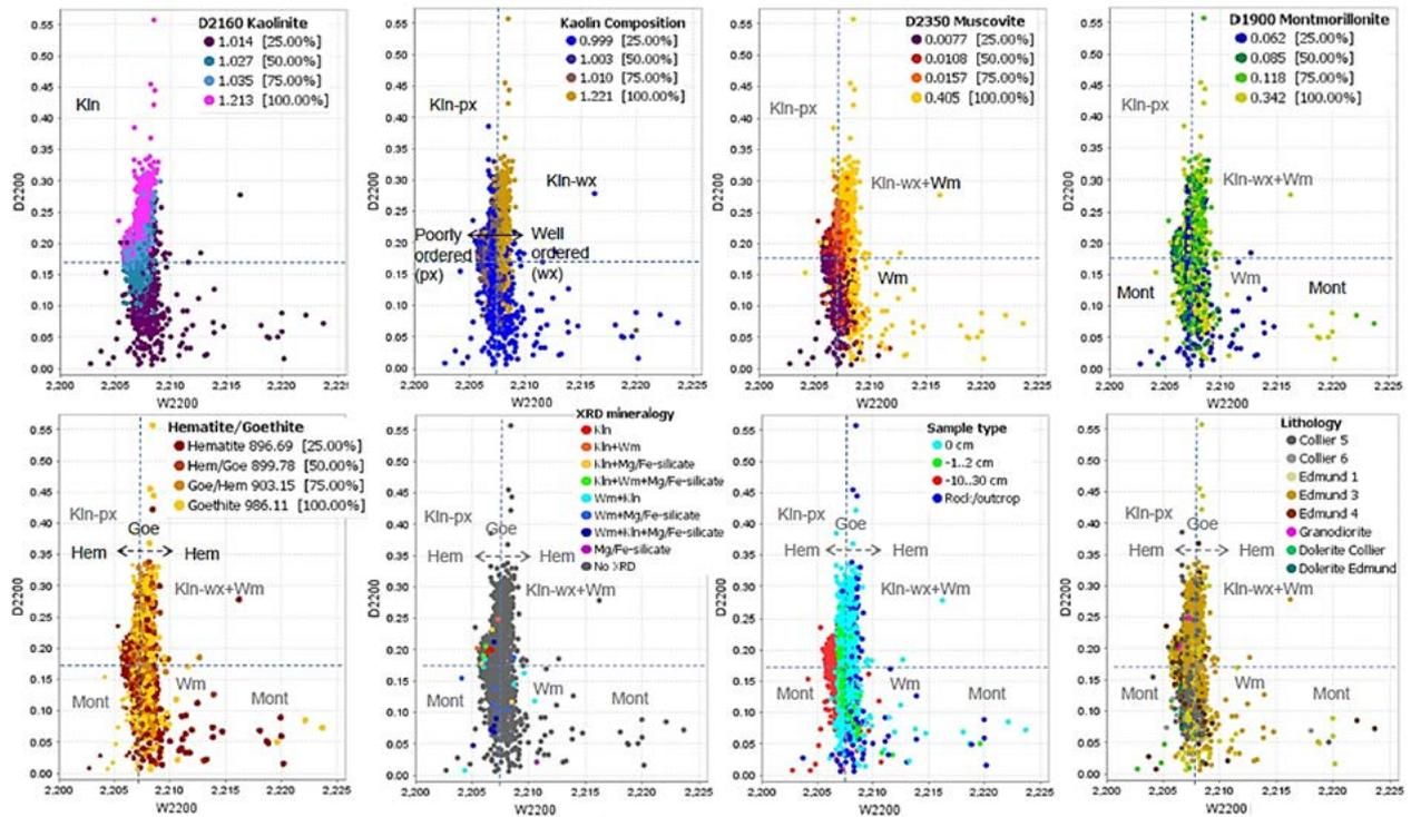
**Figure 6.** Al-clay species identification process plots using CSIRO's Geoscience products D2200/W2200, in combination with products targeting specific Al-clay minerals. "D" designates the depth of diagnostic absorption feature i.e. abundance, and "W" feature wavelength position (nm) i.e. composition. Plots are to be read from left to right and from top to bottom.
