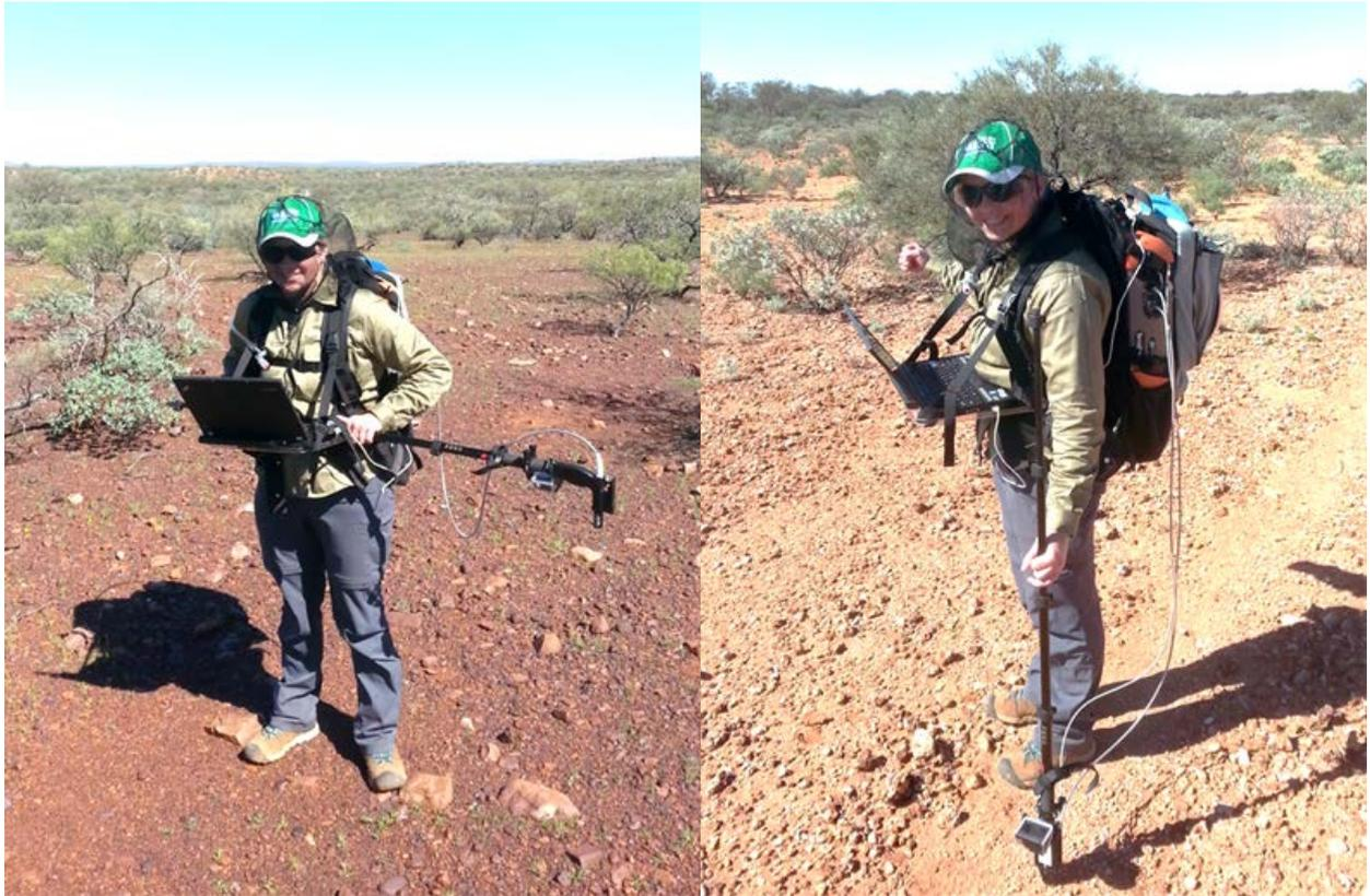
**Figure 2.** Viewing probe setup on the left and contact probe on the right. GoPro camera was attached to both probes in time-lapse and video -mode to provide continuous record of sampling (photos: Vaclav Metelka).
