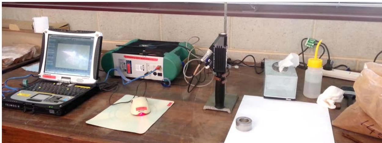
**Figure 1.** The laboratory setting at the GSWA core library for the reflectance spectra measurements from the archived regolith samples using FieldSpec3™ spectrometer together with sapphire glass container that is located on the paper in the bottom right corner of the photograph (photo: Heta Lampinen).
